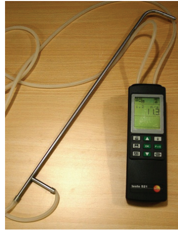
Fig. 4. Digital micro manometer TESTO 521 cooperating with Prandtl tube
