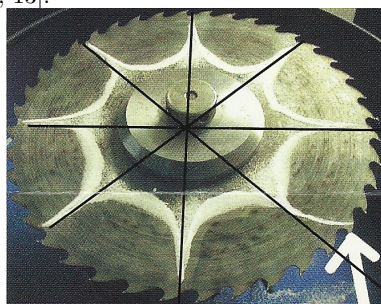
Fig. 3. Bent diameter node of the (0,4) vibration mode [12, 13]
