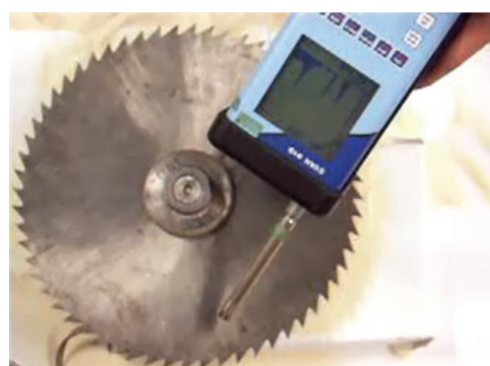
Fig. 5. FFT measurement with the Svan 912 meter
